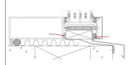
Corrected thermal break with 57mm thickness glass
