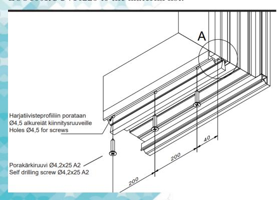
LK90X added Wall connection machining (optional) on profiles 901130 -901230 if doors fixated to facade. Instruction page 9.0, 9.1, 9.2.
